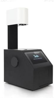
YH1100 haze meter can easily achieve ASTM D1003 non-compensation method, full light transmittance, haze test. Open sample bin can be vertically and horizontally tested to accommodate more samples to be tested. The YH1100 haze meter uses a PDF array detector to meet the CIE V( $\lambda$ )2 degree visual response. The compensation method can be used to measure the light transmittance and haze with high precision and repeatability.
